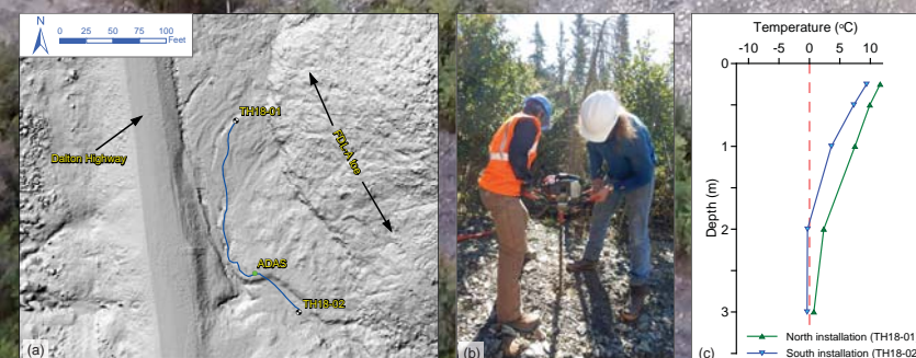
Figure 2. Overview of 2018 geomechanical instrument installation: (a) locations of borings and ADAS; (b) drilling with auger and power head; (c) preliminary temperature profile data from both borings. Background image in (a) is 2018 LiDAR DEM, collected as part of this project.
