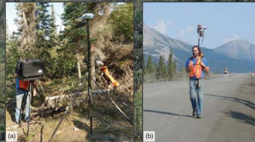
Figure 3. Acquiring 2018 LiDAR: (a) setting up base station; (b) collecting LiDAR data in back-pack mode.
